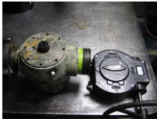
3. Ensure the gear operator is in OPEN position.
