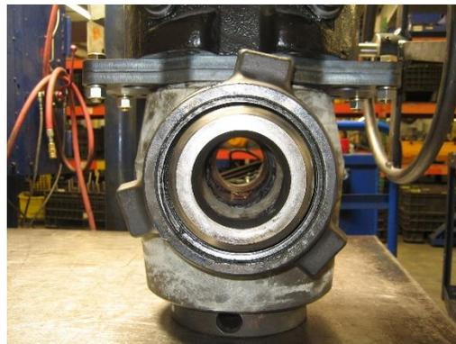
12. Set gear operator OPEN position stop. When facing the two stops, for Q-4000-S-DI gear operators this will be on the left. For Q-4000-S this will be on the right.
