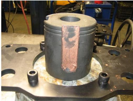
8. Carefully position the gear operator over the keyed adapter until fully seated.
