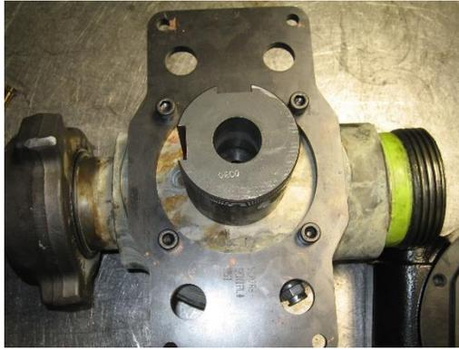
7. Lubricate the keyway and install key.
