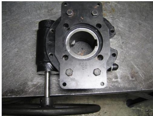
6. Install the adapter onto the valve plug. **NOTE: If the gear operator is a Q-4000-S-DI then the keyway used will need to be on the left (9 O'clock position), if the gear operator is Q-4000-S then the keyway used will need to be directly away from installer i.e. top (12 O'clock position).**
