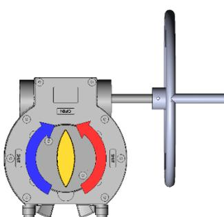
With the gear operator in the OPEN position, rotate the handwheel in the clockwise (CW) direction to close the operator. Pay attention to the rotation direction of the indicator. Gear operator identification for indicator rotation is as follows:
