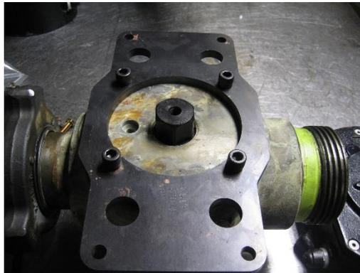
5. Lubricate the hex head bolts with thread anti-seize and install upper mounting plate to gear operator. Ensuring the longer side of the mounting plate is parallel to the gear operator shaft.
