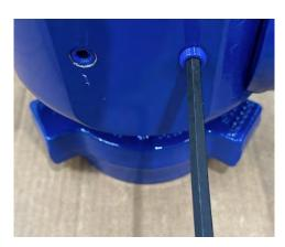
3. Attach the STA0008 service tool to the side of the valve using the 1/2" hex key. Tighten screws to 230 ft-lb.
