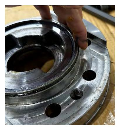
16. Place the cap on the valve such that the screw holes and keys are aligned with those on the valve body. It does not matter which direction the cap goes on otherwise.
