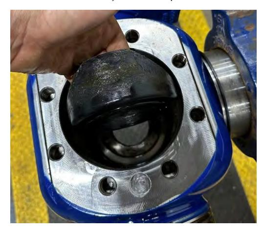
5. Rock the seat ear to ear as you push it fully into the seat pocket. The seat should be in this approximate position when it is fully seated.
