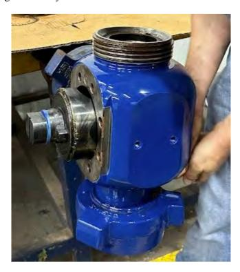
11. Once the plug has been pushed partially out, grasp it using the bore and pull straight out in one continuous motion.
