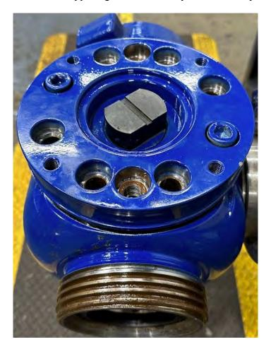
19. Using a 1/2" hex wrench or socket, alternate tightening these 2 screws to gradually bring the cap into full level engagement with the valve body. Do not use power tools for this step.
