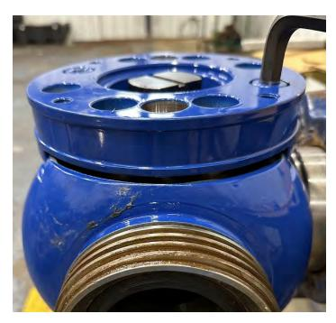
20. Once the cap is fully lowered and against the valve body face install the remaining 6 screws and tighten with hex key until fully engaged. Then use a torque wrench set to 230 ft-lbs to tighten all 8 screws in a cross pattern as shown below.
