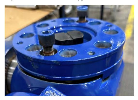
17. Apply a light coat of copper anti-seize to the screw threads. Use just enough to coat but not bury the threads.
