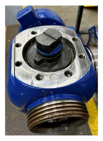
14. Place the seal backup ring onto the cap and push to the bottom of the groove. One side of the backup ring is cupped and should face the seal, but installing it in either direction is acceptable.
