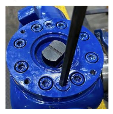
22. Rotate the valve so that the cap is down then install the handle. Make certain that the slots on the plug align with the indicators on the handle. Rotate the plug to the open position.
