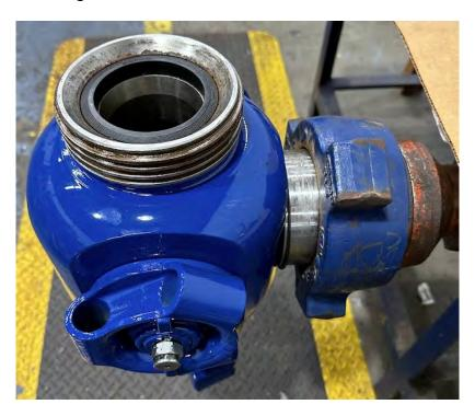
5. Rotate valve so that the handle is facing up and tighten the STA0008 wingnut to prevent rotation. Use the 2 3/16" socket to remove the lock nut. Once the locknut and handle have been removed loosen the wingnut and rotate the valve so that the cap is facing up. Retighten the wingnut.
