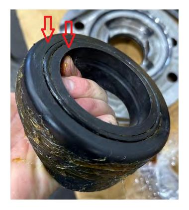
4. Lower the seat into the valve cavity with the "ears" up and down.
