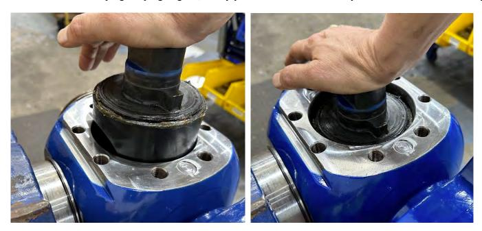
13. Rotate the plug to approximately halfway between the open and close position. There is an indicating slot on both ends of the plug that align with the flow bore. Note in the photo below the plug orientation to the end connections.
