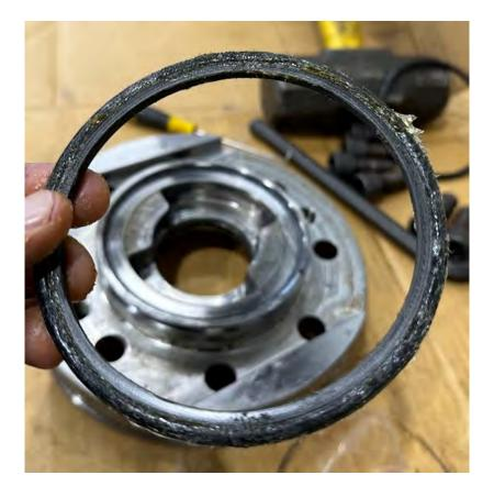
9. Press the seals onto each end of the plug being sure they are firmly seated. There should be enough grease present to keep the bottom seal from falling off.
