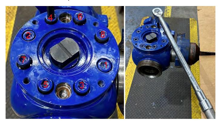
21. Replace the plastic plugs to keep the jack screw threads protected from the elements. Do not overtighten or the plastic threads will fail.
