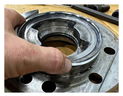
15. Apply a light coat of plug valve grease on the cap seal then place it into the groove on top of the backup ring. Go around the seal with your finger to evenly distribute it in the groove.
