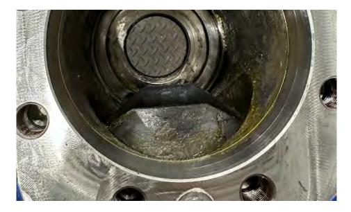
6. Now rotate the seat by hand until it is aligned with the valve cavity. Adjust the seat rotation until the standoff is even on both sides of the seat [blue arrows]. Repeat this process for the second side.
